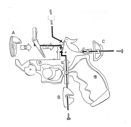
The release lever should have the pivot points in the center of the arm (the outside of the L/R sides) drilled out to allow a screw to go through. Make sure all excess flashing is trimmed from this part as well. It should move against the sides of the grip without binding.
