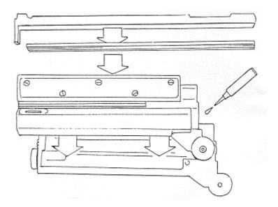
Now you should Epoxy the long metal support bar into the channel in the bottom of the top sight rail. Let the epoxy cure for about 20 minutes or so and then sand off any excess. Take the *White Metal Locking Bracket* and test it to make sure it will fit. You may need to remove some small amount of material with a hobby knife for it to fit correctly.
