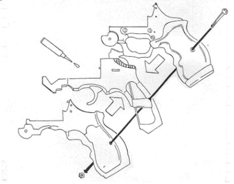
Originally, I suggested gluing the trigger parts into the outer grip halves. This step is actually *not* needed as the grip bolt keeps everything tightly in place. Also, in the event that I release a replacement for the trigger unit (Which I'm hoping to do sometime in the future) you will still be able to remove and replace the trigger.
